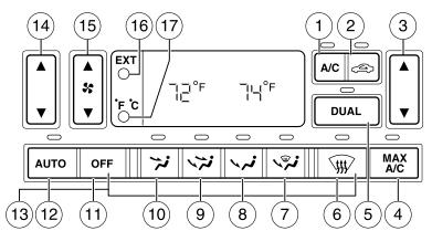
1. **A/C control:** Press to turn on the air conditioning. Press again to turn off the air conditioning. Use
